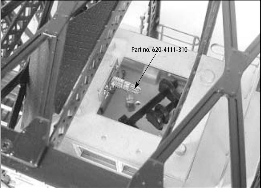
Figure 8. Control cabin interior lamp
