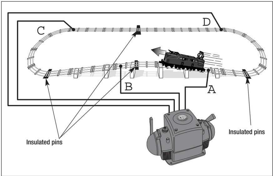
Figure 10. Control of various track blocks
