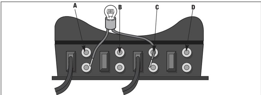
Figure 8. Checking the phase of your PowerHouse Power Supplies
