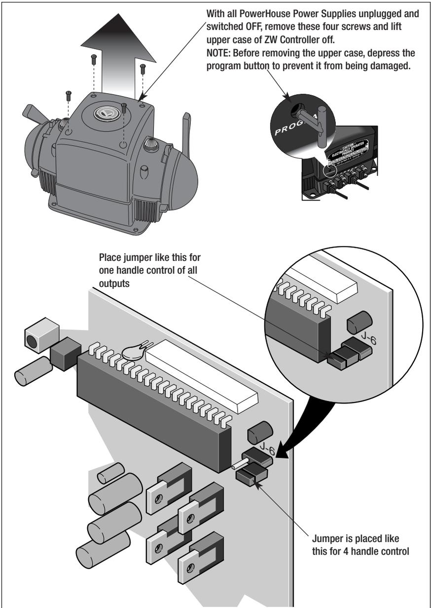
Figure 9. Setting the jumper
