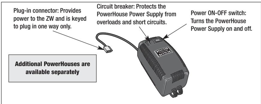
Figure 1. Features of the PowerHouse Power Supply
