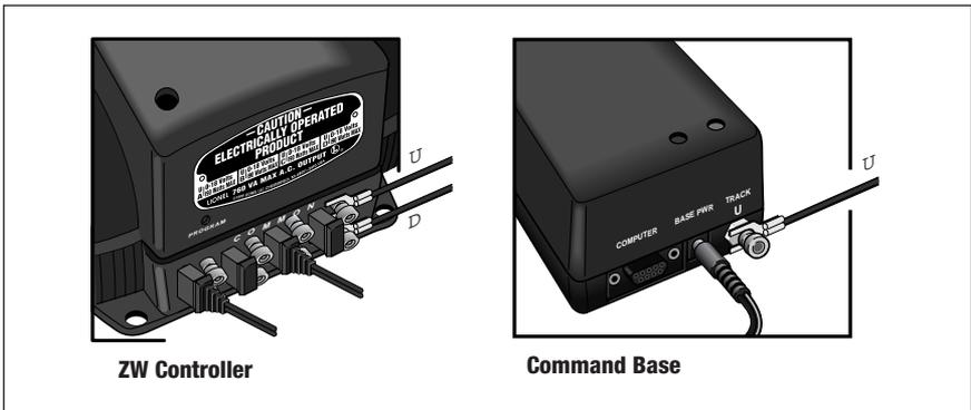
Figure 5. Command Base connection
