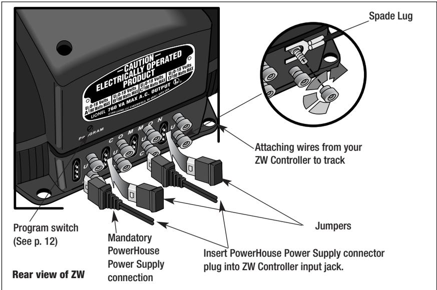
Figure 3. PowerHouse connections
