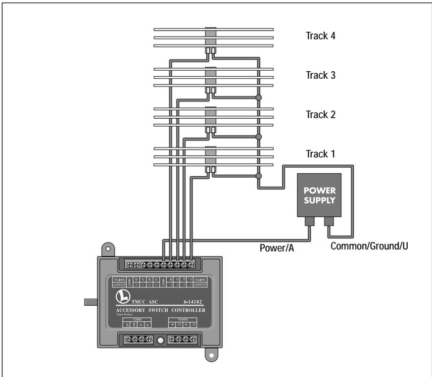
Figure 11. Wiring blocks of track in conventional mode
