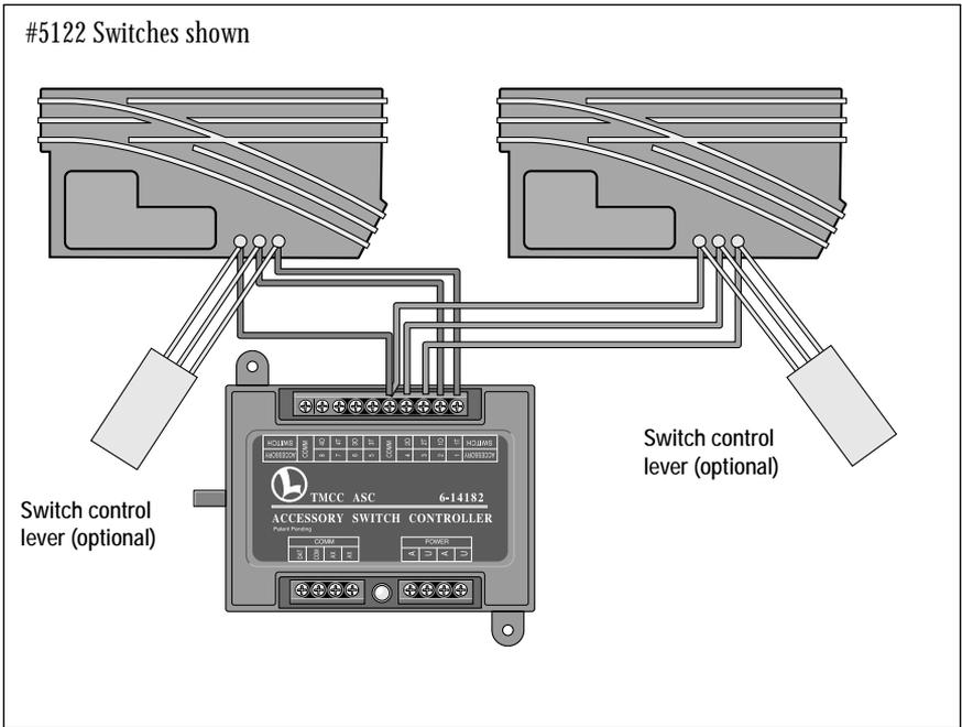
Figure 12. Example of coil switch wiring
