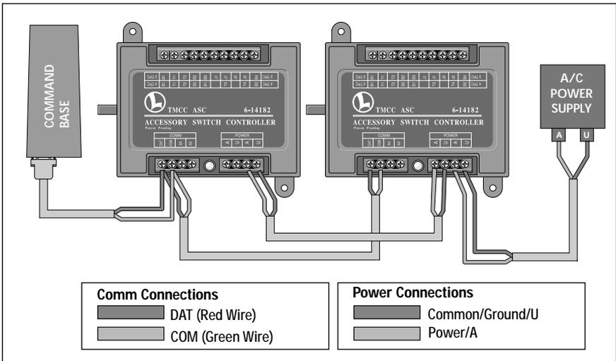
Figure 2. Connecting additional TMCC products in a “daisy chain”
