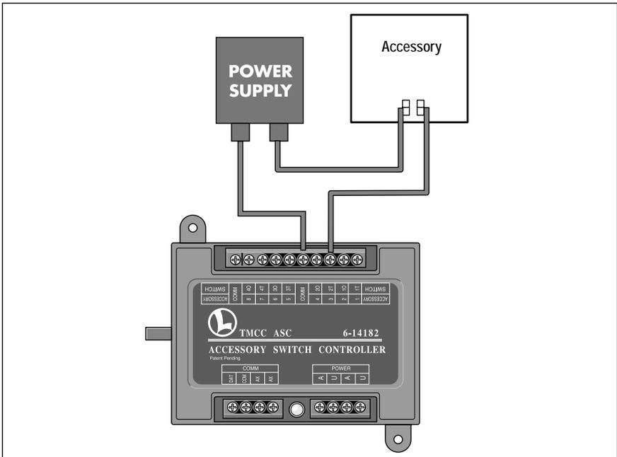
Figure 3. Example of accessory wiring
