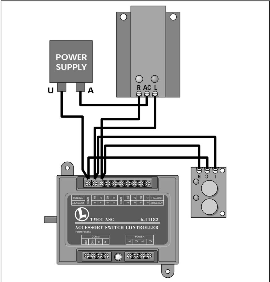
Figure 17. DZ-1000 Switch wiring
