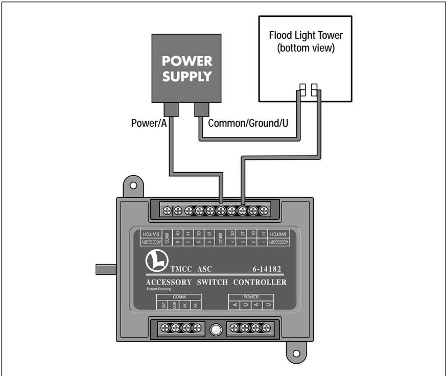
Figure 6. Floodlight Tower wiring
