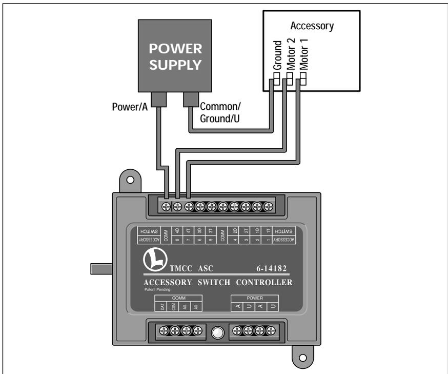
Figure 4. General wiring for accessories with multiple motors or lights
