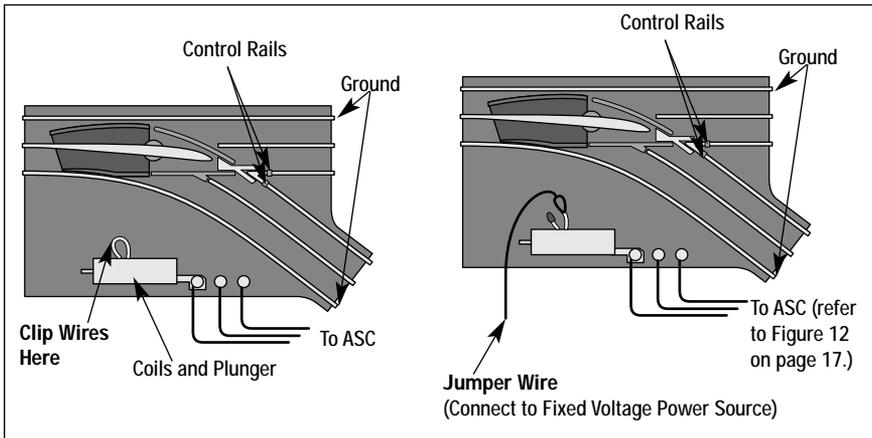
Figure 13. Wiring Lionel O-27 gauge switches
