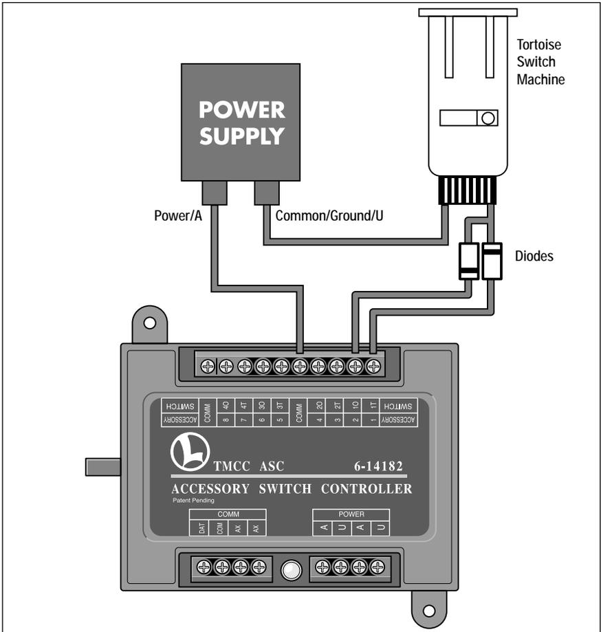
Figure 14. Tortoise switch wiring
