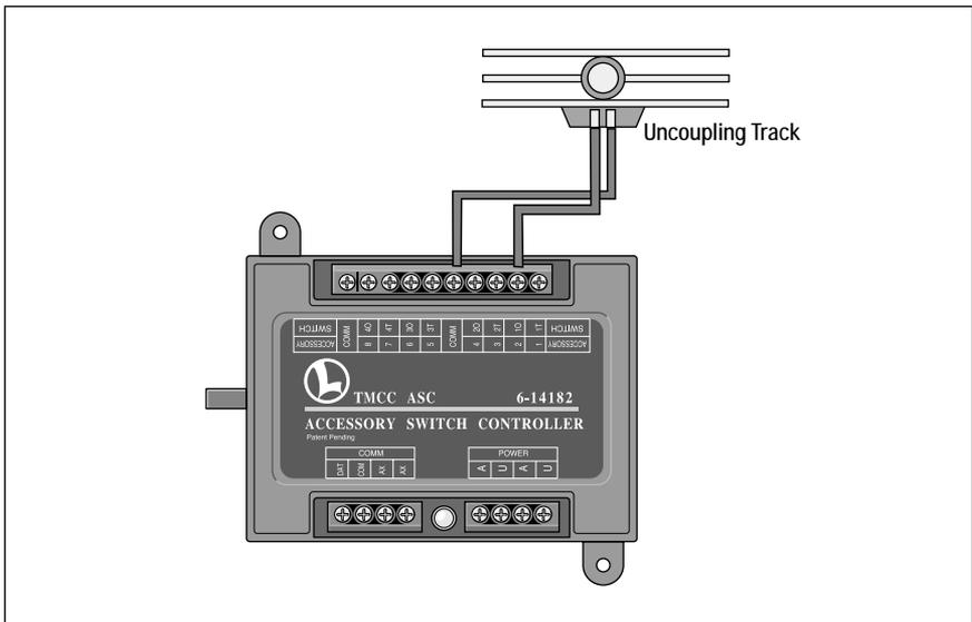
Figure 8. Uncoupling Track wiring
