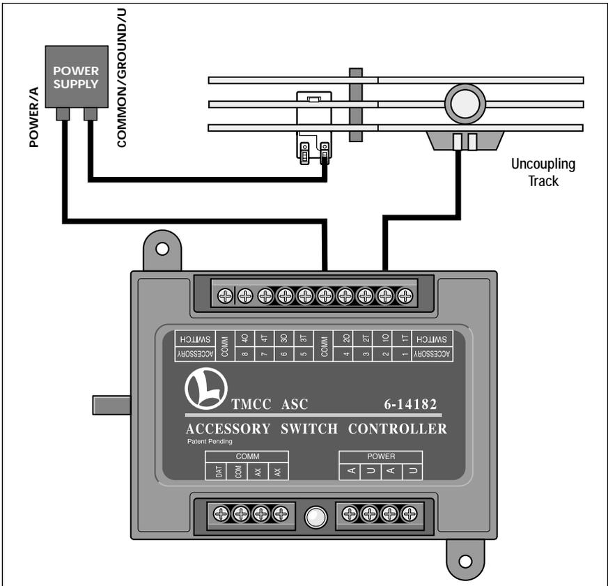
Figure 9. Uncoupling Track wiring using fixed voltage
