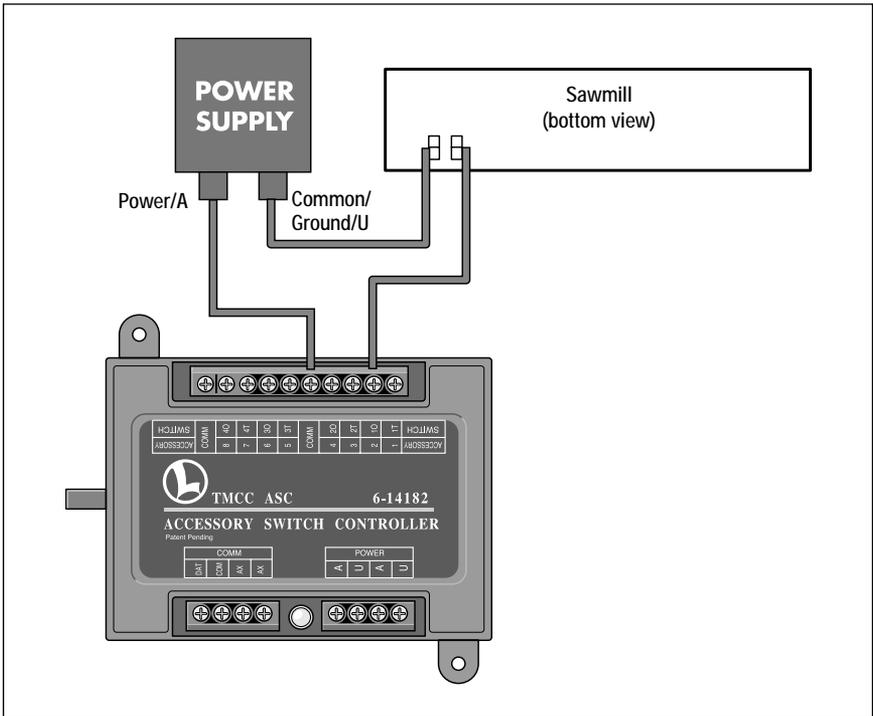
Figure 7. Sawmill wiring
