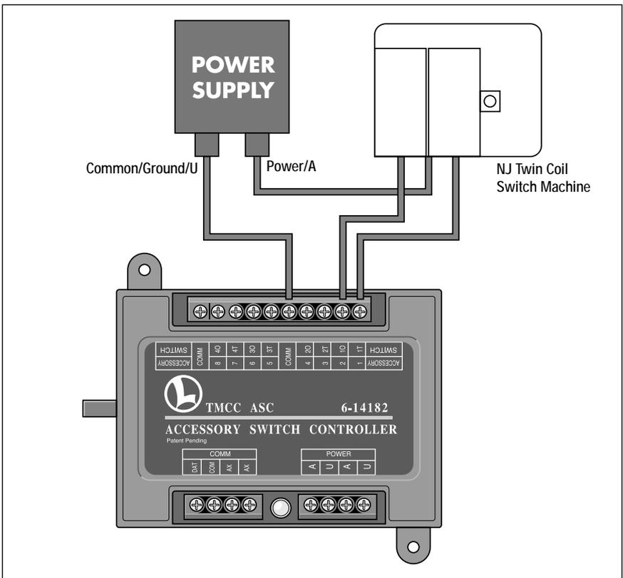
Figure 15. NJ Twin Coil Switch wiring
