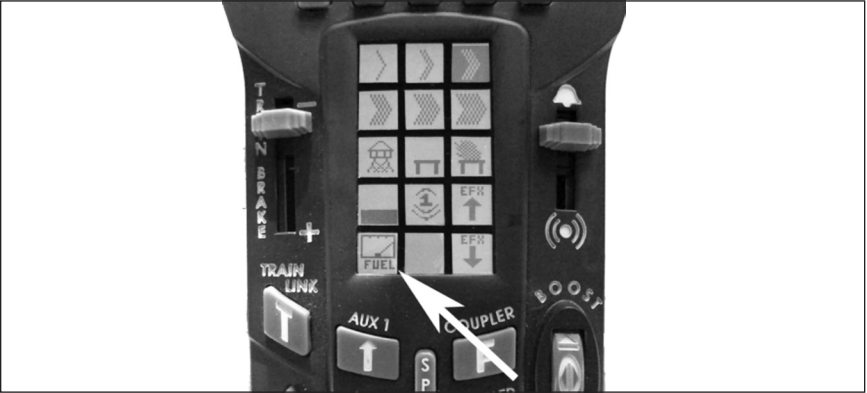
Figure 12. The IRV2 enables a fuel level displayed on a LEGACY CAB-2 remote
