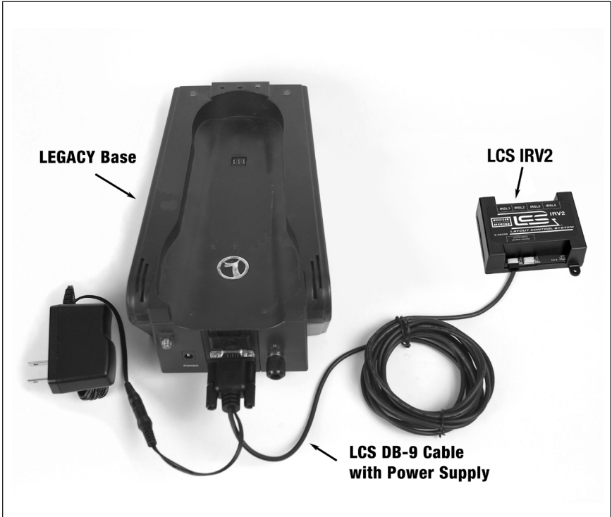
Figure 5. A sample LCS system with the IRV2 and a LEGACY Base
