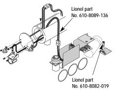
the four screws taking care to not pinch any wires during reassembly.
