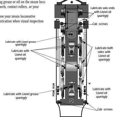
Do not lubricate your locomotive's electric motor.. It has been pretested and all the necessary moving parts have been sufficiently lubricated for life at the factory and should run smoothly for many years to come. If
