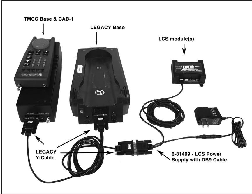
Figure 6. Installing LCS with Legacy AND TrainMaster Command Bases
