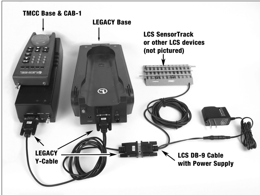
Figure 7. A sample LCS system with SensorTrack, a LEGACY Base and an original TMCC Base.”
