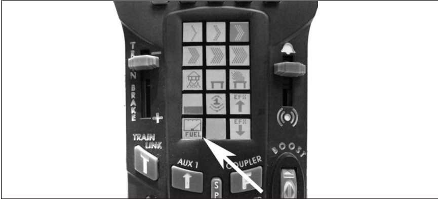
Figure 11. SensorTrack enables a fuel level displayed on a LEGACY CAB-2 remote
