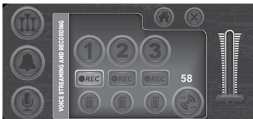
Figure 16. While recording, the REC button will turn blue and a 60 second timer will count down.
